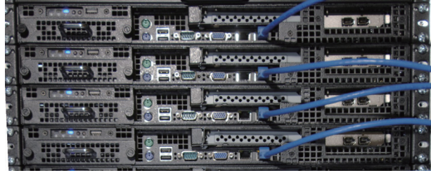
Figure 3: Front details of Opteron nodes
