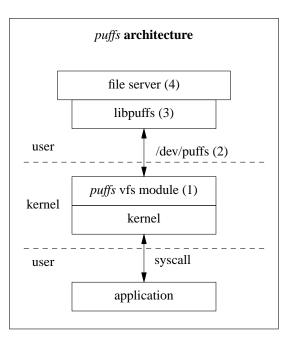
The vfs layer is made up of two separate interfaces: the actual virtual file system interface and the vnode interface. The former deals with calls involving file system level operations, such as mount and unmount, while the latter always involves an operation on a file; the vnode or virtual node is an abstract, i.e. virtual, representation of a file.
