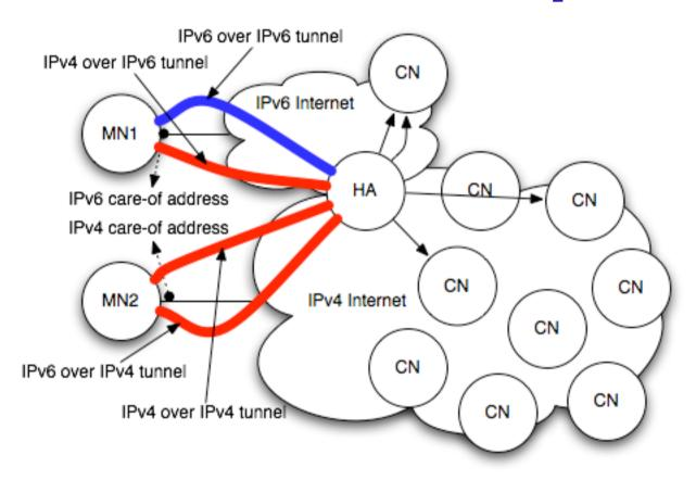
MIPv6 provides IPv6 over IPv6 tunnel (blue line) DSMIPv6 provides other tunnels (red line)
